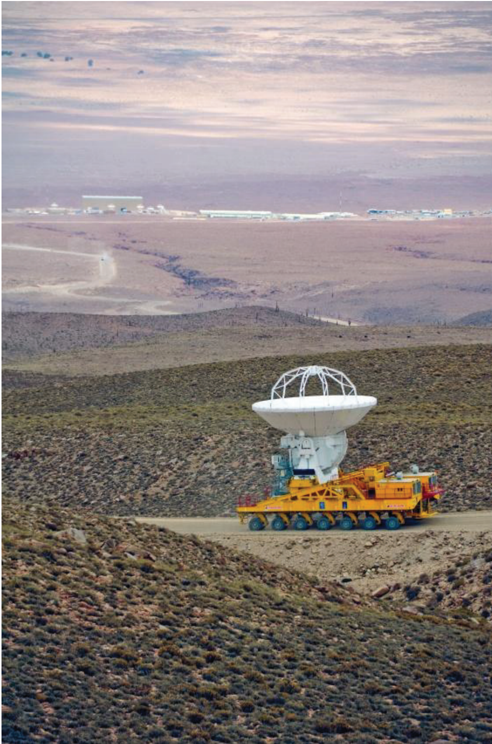
An ALMA antenna en route from the Operations Support Facility to the plateau of Chajnantor for the first time. The ALMA transporter vehicle carefully carries the state-of-the-art antenna, with a diameter of 12 metres and a weight of about 100 tons, on the 28 km journey to the Array Operations Site, which is at an altitude of 5000m. Credit: ALMA (ESO/NAOJ/NRAO)
