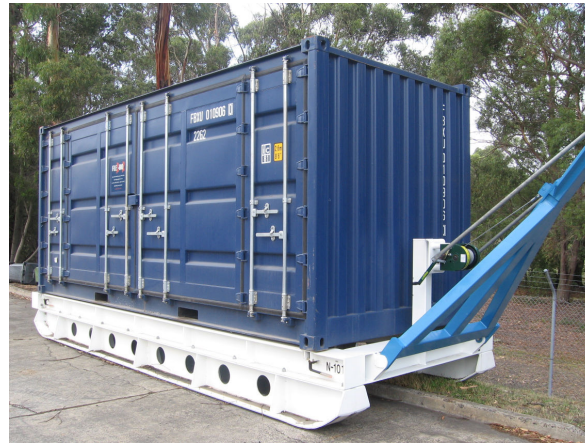
Fig. 5. 20 tonne sled (this one without suspension). 3 x 7m bed, tare mass 7 tonnes.
