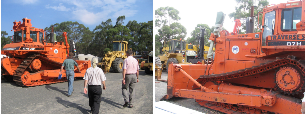
Fig. 4. Caterpillar D7 traverse-type tractor, at AAD for refurbishment.
